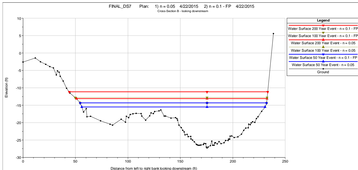
Figure 10 - HEC-RAS calculated water surface results for the 50, 100, and 200 year events at cross-section B with a low ( n=0.05 across channel) and high ( n=0.05 in channel and 0.1 in floodplain) roughness senerio. Depicted facing downstream, this is the middle of three cross-sections in the modeled reach.
