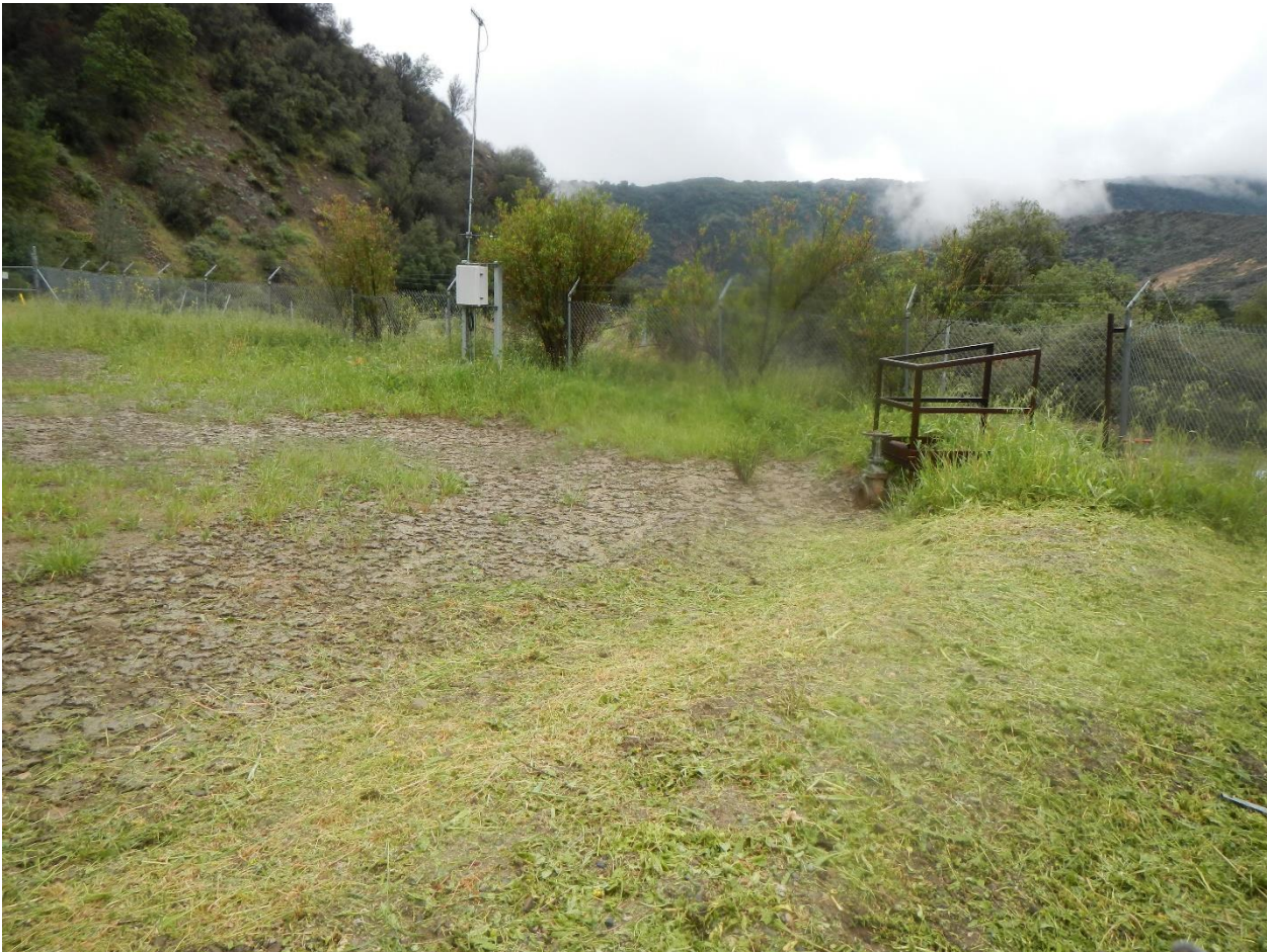
Picture 3 – Western edge of Drill Site No. 7 facing the drain. No ponding near the drain. Silts and clays appear cracked from swelling and shrinking due to moisture accumulation and evaporation. Picture taken on April 7, 2015 at 4:12 pm
